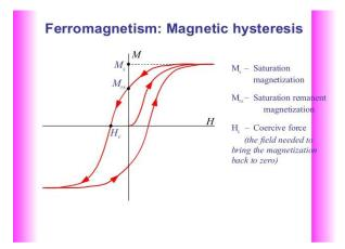
Initially, as H increases, M increases until a saturation point Ms is reached. When H is decreased from the saturation point, M does not decrease to the same value it had before: rather, it is higher on the curve of the decreasing field. This is called hysteresis.
