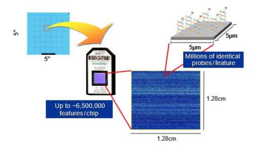
These GeneChip microarrays are a fusion of the technology of the semiconductor industry with life sciences – this is why these arrays are called "chips". The chips are manufactured on wafers. These wafers are 5-inch-by-5-inch pieces of glass. You can get anywhere from 49 to 900 individual chips out of each wafer, depending on the overall size of the final chip to be made
