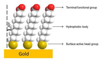
Surfaces with micron and nanopatterns of SAMs are interesting since they allow the creation of metallic hybrid circuits where biomolecules can be selectively attached (and released) to patterns of gold. Different methods exist for creating micro and nanopatterns of SAMs, such as microcontact printing ( $\mu$ CP), nanocontact printing (nCP), conventional lithography and Dip Pen Nanolithography.
