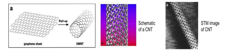
Nanotubes are formed by rolling up a graphene sheet into a cylinder and capping each end with half of a fullerene molecule.
