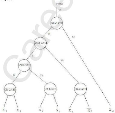
Now, let us consider a part of the circuit as shown below: Here we have two wires  $y_1$  and  $y_2$  feeding into an or gate and the output wire is  $y_5$ .
