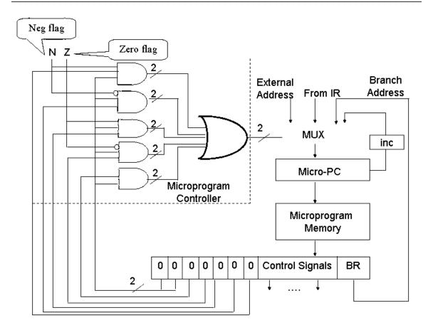
If a branch instruction is encountered within the microprogram hardwired logic selects the branch address as the source of micro-PC using 4 to 1 mux. This hardwired logic caters for all branch instructions including branch if zero.
