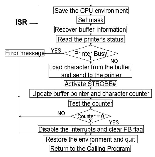
These values become part of the binary file and are then loaded into the memory when the binary file is loaded and executed. In response to a hardware interrupt or the software interrupt **int**, the control unit of the FALCON-A CPU will pick up the address of the first instruction in the ISR from memory location 2, and transfer control to it. This effectively means that the behavioral RTL of the **int** instruction will be as shown below:
