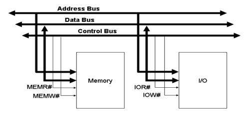
address bus, the data bus and the control bus. These three buses are being applied to the I/O module in this figure. At the bottom, we see a set of data, status and control lines from each "device interface logic" block. Each of these sets connects to a peripheral device. I/O decoding logic is also shown in this figure
