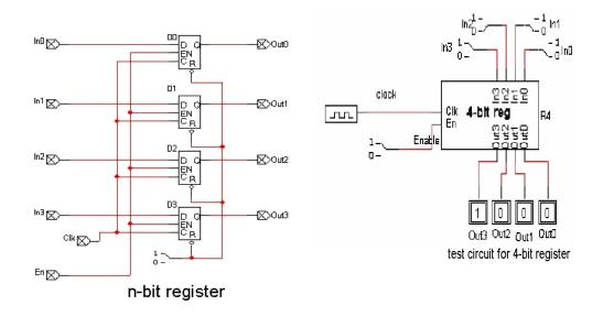
The next figure shows the symbol of a 4-bit register used for an integrated circuit. In0 through In3 are the four input lines, Out0 through Out3 are the four output lines, Clk is the clock input, and En is the enable line. To get a better understanding of this register, consider the situation where we want to store the binary number 1000 in the register. We will apply the number to the input lines, as shown in the figure given.
