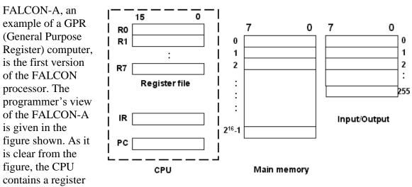
file of 8 registers, named R0 through R7. Each of these registers is 16 bits in length. Aside from these registers, there are two special-purpose registers, the Program Counter (PC), and the Instruction Register (IR). The main memory is organized as  $2^{16} \times 8$  bits, i.e.  $2^{16}$  cells of 1 byte each. The memory word size is 2 bytes (or 16 bits). The input/output space is 256 bytes (8 bit I/O ports). The storage in these registers and memory is in the big-endian format.
