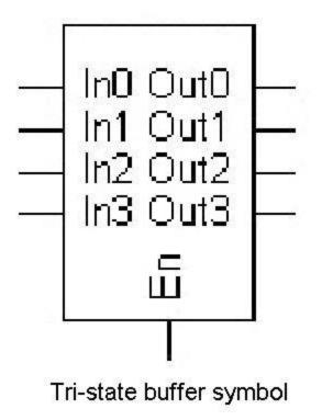
We can see that when the enable input (or the control input) c is low (0), the output is high impedance Z. The symbol of a 4-bit tri-state buffer unit is shown in the figure. There are four input lines, an equal number of output lines, and an enable line in this unit. If we apply a high on the input 3 and 2, and a low on input 1 and 0, we get the output 1100, only when the enable input is high, as shown in the given figure.
