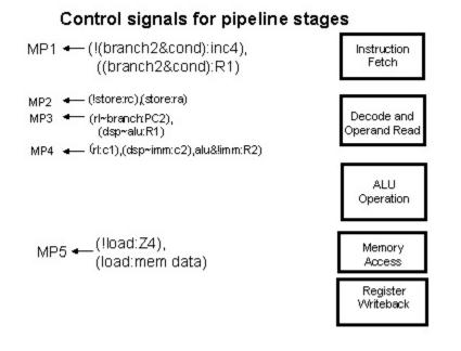
The multiplexer MP5 is used to decide which value is transferred to be written back to the register file. If the load signal is activated data from memory is transferred to Z5, however if the load signal is not activated then data from Z4 (which is the result of ALU) is transferred to Z5 which is then written back to the register file.
