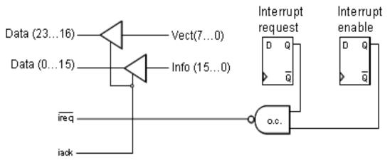
module. Once the correct module is identified, the CPU branches to a device service routine which is specific to that particular device.
