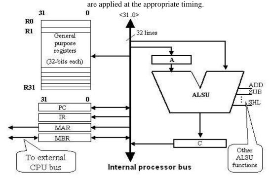
As will be obvious, control signals need to be applied to the ALSU, based on the decoding of the op-code field of an instruction. The given table lists these control signals:
