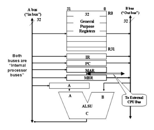
**Structural RTL for the 'sub' instruction using the 2-bus data path implementation** Next, we look at the structural RTL as well as the control signals that are issued in sequence for instruction execution in a 2-bus implementation of the data path. The given table illustrates the Register Transfer Language representation of the operations for carrying out instruction fetch, and execution for the sub instruction.
