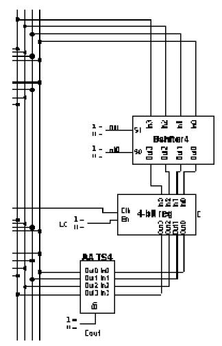
Shift operation using Barrel Shifter
