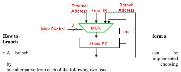
This scheme provides flexibility in choosing branches as we can form any combination of conditions and addresses.
