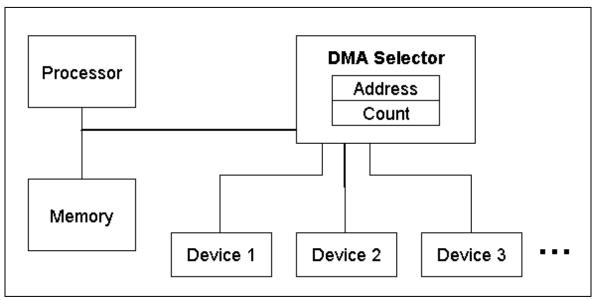
It is the DMA controller that can do block transfers for several devices at once.
