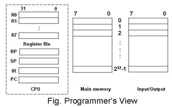
FALCON stands for First Architecture for Learning Computer Organization and Networks. We are already familiar with our example processor, the FALCON-A, which was the first version of the FALCON processor. In this section we will develop a new version of the processor. Like its predecessor, the FALCON-E is a General-Purpose Register machine that is simple, yet is able to elucidate the fundamentals of computer design and architecture.
