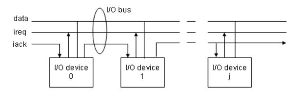
As we said that the previous device should not have generated an interrupt, that means its interrupt was not enabled and therefore, it passes on the acknowledge signal from its output to he next device.
