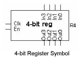
On the leading edge of the clock, the number will be stored in the register. The enable input has to be high if the number is to be stored into the register.
