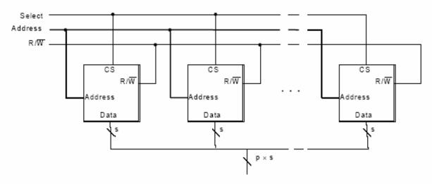
P chips expand word size from s bits to p x s bits.
