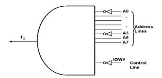
To make things simple, we use a circle (or a bubble) to indicate an inverter, as shown .Since this is a 16-bit output port, we will use two 8-bit registers to capture data from the FALCON-A's data bus. The output of the SAD will be connected to the enable inputs of the two registers. The D-inputs of the registers will be connected to the data bus and the Q outputs of the registers will be connected to the peripheral device.
