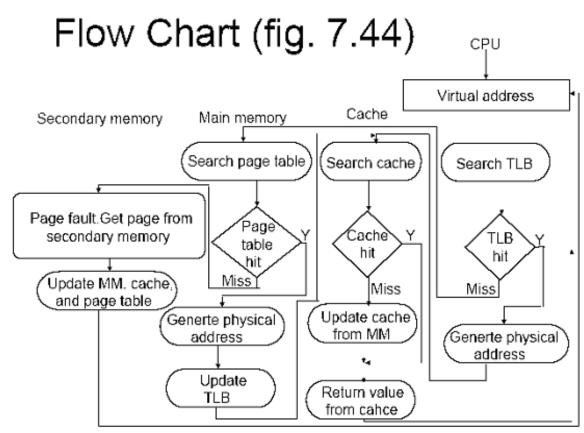
To reduce the work load on the CPU and to efficiently use the memory sub system, different methods can be used. One method is separate cache for data and instructions. **Instruction Cache:** It can be implemented as a Translation Lookaside buffer. **Data Cache:** In data cache, to access a particular table entry, it can be implemented as a
