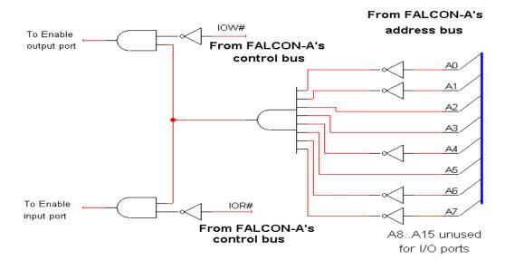
FALCON-A's Address Decoder for an I/O Port at the Address 2Ch
