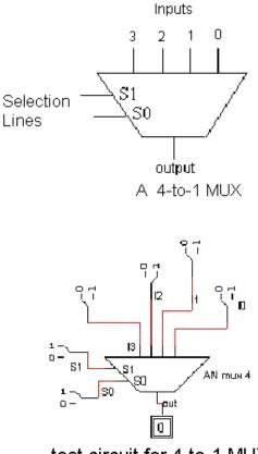
test circuit for 4-to-1 MUX
