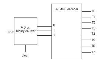
analogous to the clock cycles in the actual processor. A possible implementation of the timing step generator is shown in the figure.
