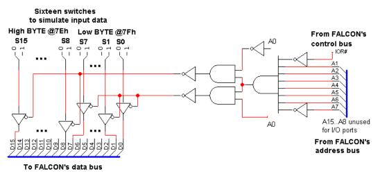
A 16-bit parallel input port for the FALCON-A at address 7Eh and 7Fh
