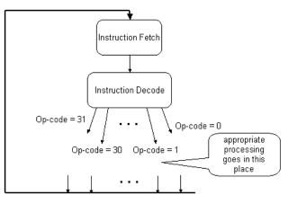
same process is repeated until the instruction with op-code 31 would reach and halt the system.
