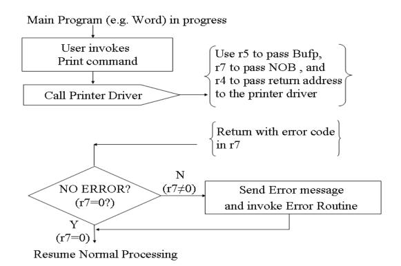
document is placed in a buffer by the word processor. This buffer is usually present somewhere else in the memory. The responsibility of the calling program is to pass the number of bytes to be printed and the starting address of the buffer where these bytes are stored to the printer driver. The calling program can also be called the main program.
