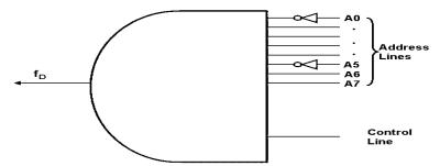
Next, we look at the relevant control signals. The only signal which should be used in this case is IOW#. A logic 0 (zero) on this line indicates that it is active. Thus, it should be inverted before being applied to the input of the SAD.
