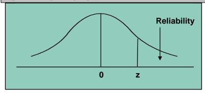
Product failure due to wear out can be determined by using normal distribution. From our knowledge of statistics we already know that the statistic table for a standardized variable Z represents the area under the normal curve from essentially from the left end of the curve to a specified point z, where z is a standardized value computing use
