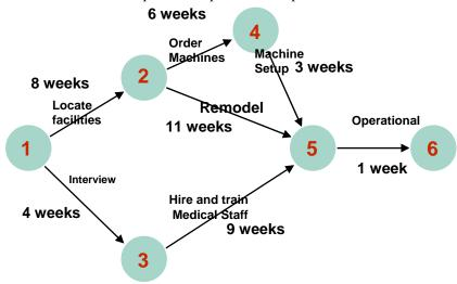
The activities from locating the facility to making the hospital fully are represented in the form of a network diagram. The student should try to write down the activities along with the activity description then try to draw the network diagram using both the activity on node and activity on arrow as practice.
