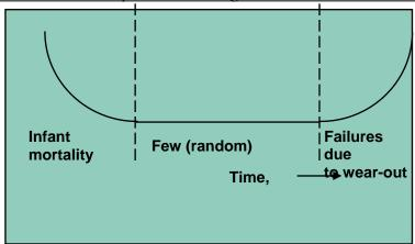
The figure above shows a bathtub shape and thus rightly is referred to as the Bathtub curve. On the Y axis we represent the Failure rate and on the X axis we represent the Time. A careful look at the graph would help us to identify the three phases
